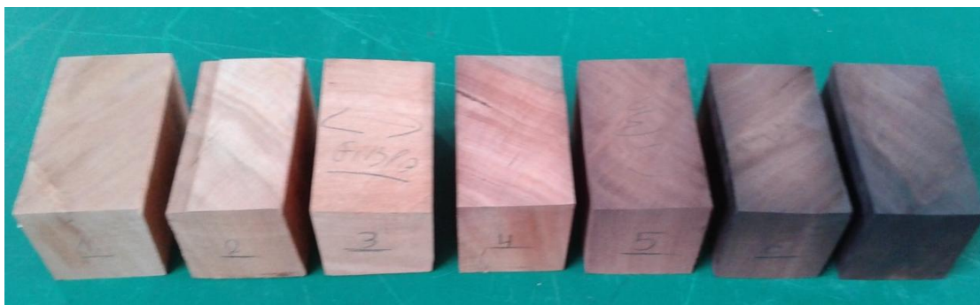
Figure 4. Specimens after thermal treatment. Shown 1 (at left) to 7 (at right).
