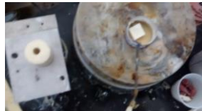
Figure 3: Elastomer template and wax being melted.
