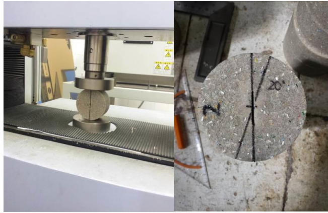
Figure 4. a) Experimental setup; b) Sample with positioning markings for 20 degrees
