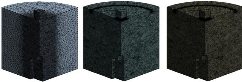
Figure 5. Mesh generated in the three geometries. Maximum element size of 2 cm in the regions of interest
