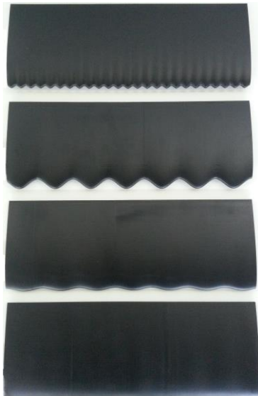
Figure 2. The set of four airfoils for profile NACA 0012.
