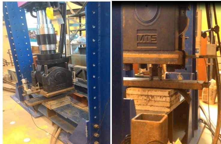
Figure 4.(a) Equipment used in the double lap joint test (b) Setup of the test body during the experiment.
