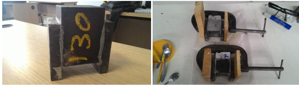
Figure 3. (a) Test body after curing process (b) Application of pressure to test bodies during curing process.
