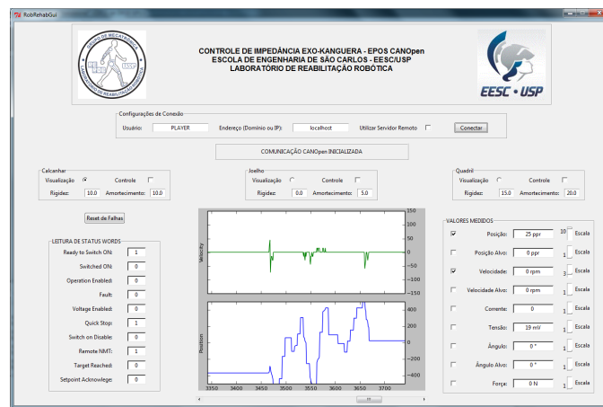
Figure 4: Therapist GUI, built in TK, showing the available controllers and data visualization graphs and boxes.
