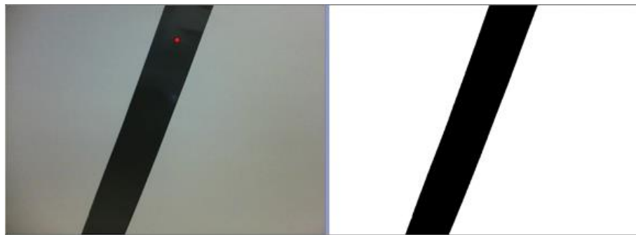
Figure 5: Location of the line center (red dot in Fig. to the left) and binary image using the experimental thresholding method (right)
