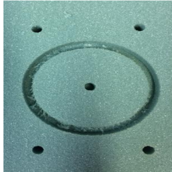
Figure 7. PVC part with five holes and one circular slot that was machined using the STEP-NC standard
