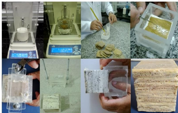
Figure 2. Manufacturing process of composite test specimens under study
