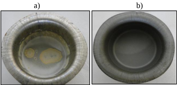
Figure 3 - Specimens after durability test. (a): Cups with tin coating; (b): Cups with organometallic coating.
