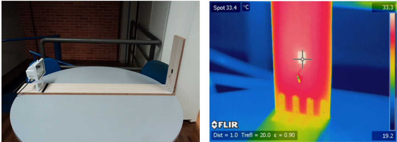
Figure 4. Apparatus to evaluate the generation of electricity and heat by halogen lamp (left side) and thermal imaging of PV cell (right side).
