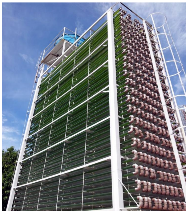
Figure 1 - Compact tube photobioreactors developed by NPDEAS-UFPR
