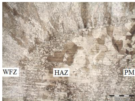
Figure 5 – Microstructure of the region of transition between Welded Fusion Zone and Parent Metal.
