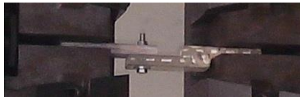
Figure 4. Overview of the apparatus and the composite plate in the grips of the testing machine.
