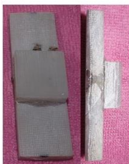
Figure 2. Test piece with joint-adhesive ready for testing.
