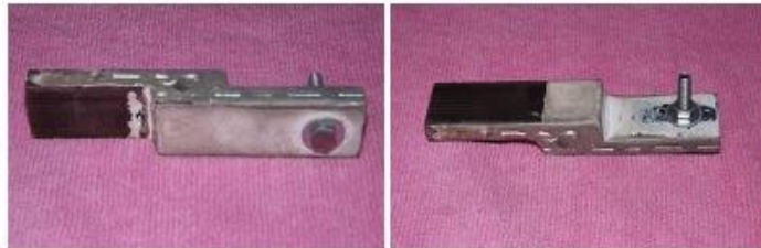
Figure 3. Views of the fixing apparatus to fix the pinned joint in the testing machine.
