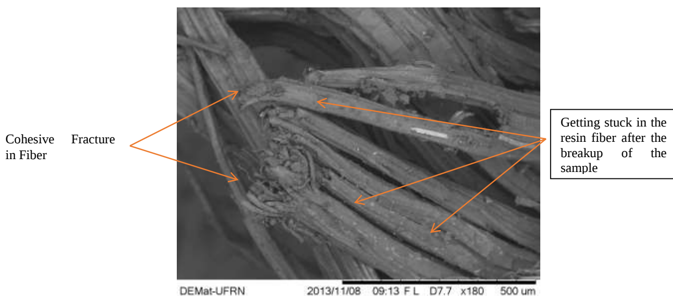
Figure 6. Composite without immersion (dry) (SEM held at specimen fracture)
