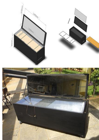
Figure 1. Solar oven proposed in test in the Solar Energy Laboratory/ UFRN.
