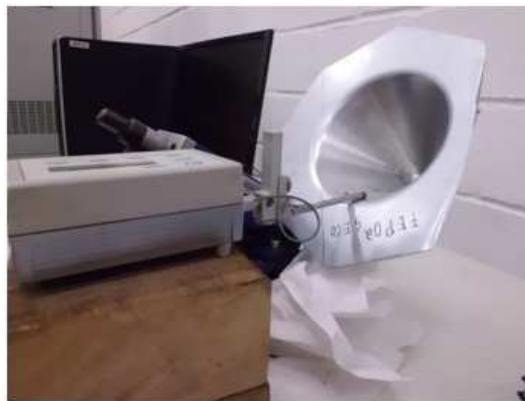
Figure 5. Roughness analysis done with profilometer.
