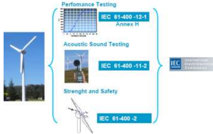
Figure 1. Tests for certification of a wind turbine (Alé, 2012).
