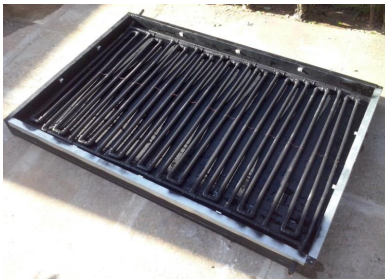
Figure 1. Solar collector during its manufacturing process.
