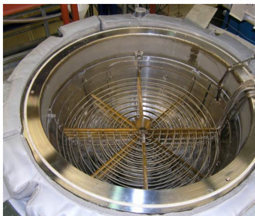
Figure 2. View of the LIVE-3D vessel with heating coils
