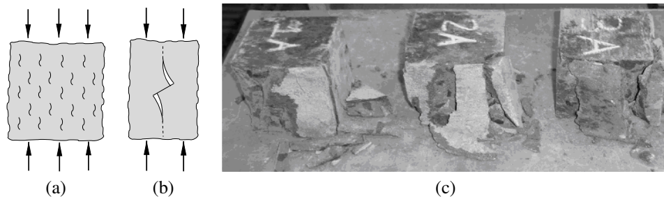
Figure 4. Schemes that illustrate the damage process in quasi-brittle materials under compression: (a) fissures appear in loading direction, (b) self-organization and propagation at an angle and the sliding dissipation process begins to be dominant. (c) Experimental results for the case without lateral restriction in both ends.
