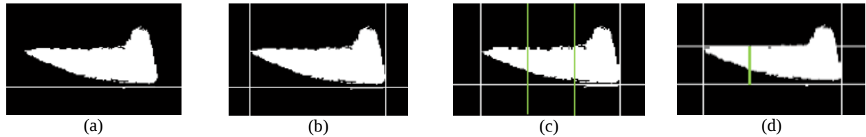
Figure 4: Image processing. a) Delimitation of workpiece. b) Horizontal Limits. c) Zone for measurement of weld bead reinforcement. d) Reinforcement measure.
