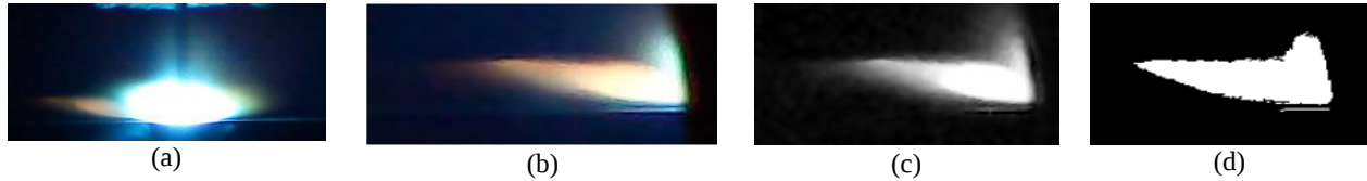
Figure 3: Image acquired by the webcam. a) With strong influence of the arc light. b) Image acquired and cropped. c) Image in grayscale and median filter. d) Image binarized.
