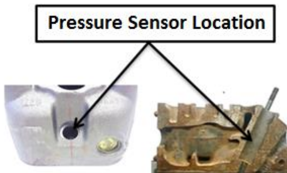
Figure 2. Position of the pressure sensor in the engine head
