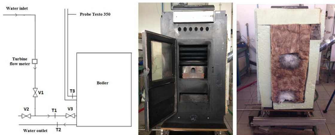
Figure 2. Installation scheme and boiler photo before and after insulation
