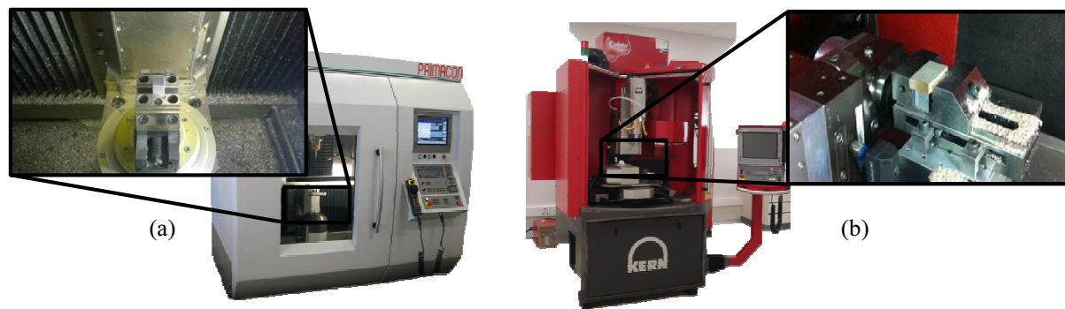
Figure 2. Set-up of micro-milling centers: (a) Primacon PFM 4024-5D and (b) KERN Evo
