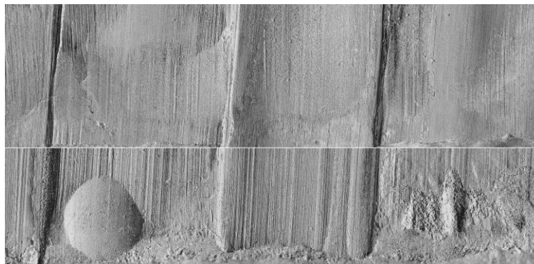
Figure 7. Images of test-fired projectiles from the same gun, at the top of the image a CS6 (G-JHP) and at the bottom a CS1 (LRN).
