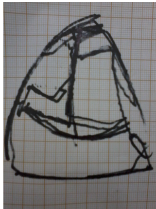
Figure 6. 3-RRR planar parallel robot workspace drawn in second approach
