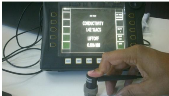
Figure 8 - Conductivity and thickness (lift-off) reading in the sample with bond coat deposited on Inconel 718.
