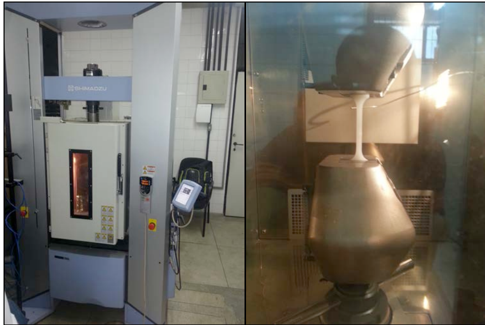
Figure 2. PVDF tensile test
