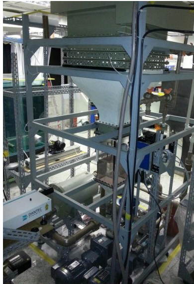
Figure 4. Vertical water tunnel with PIV system aligned
