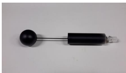
Figure 5. Sphere used to validate the vertical water tunnel
