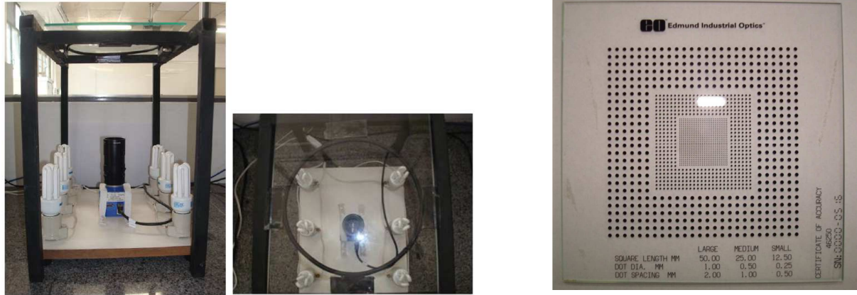
Figure 4. Structure for image acquisition (a) Front view (b) Top (c) Calibration standard
