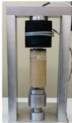
Figure 2. Coil + Levitated Mass
