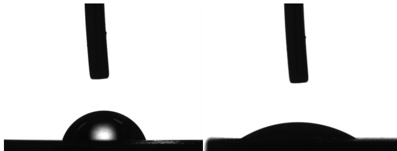
Figure 5. Comparative analysis of the contact angle in titanium surface; the right, titanium machined and polished; the left, modified titanium plasma.
