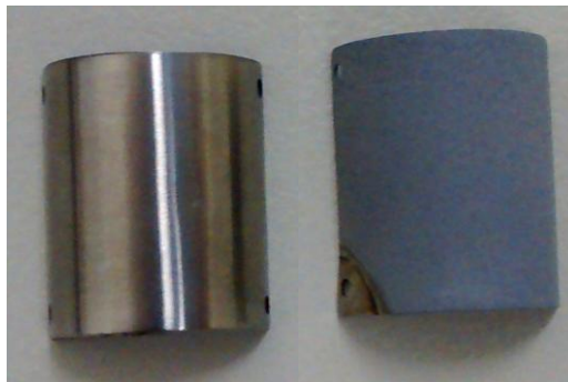
Figure 3. Pictures from titanium implant with medical grade II; A. Reference Material and B. Implant treated with electrolytic plasma.
