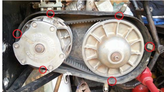
Figure 3 - Thermocouples positions using to measure the temperature in the CVT pulleys
