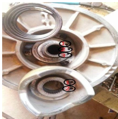
Figure 4. Setting the pulley spring positions moved from CVT Polaris P90
