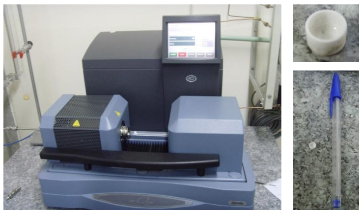
Figure 1. Simultaneous thermal analysis system installed on Combustion Laboratory and Carbon Capture LCCC/ FEG-UNESP, in Guaratinguetá/ SP.
