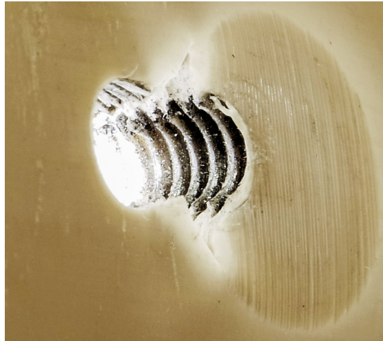
Figure 2. Thread marks in specimen 2 (M6) after testing
