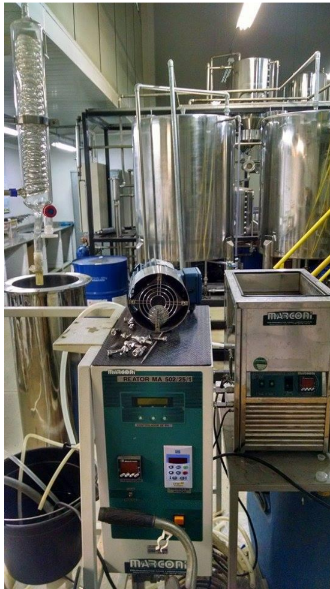
Figure 2. Reactor utilized for the extraction of fatty acids by saponification process.
