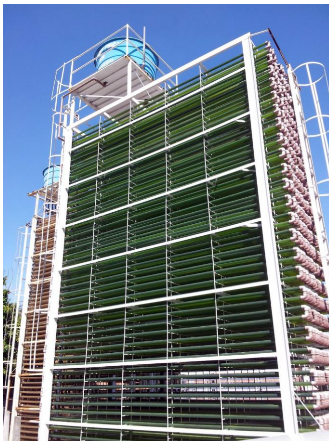
Figure 1. Photobioreactor where the microalgae Scenedesmus sp. was cultivated.
