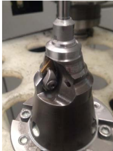
Figure 3. Cutting tool with PCBN insert
