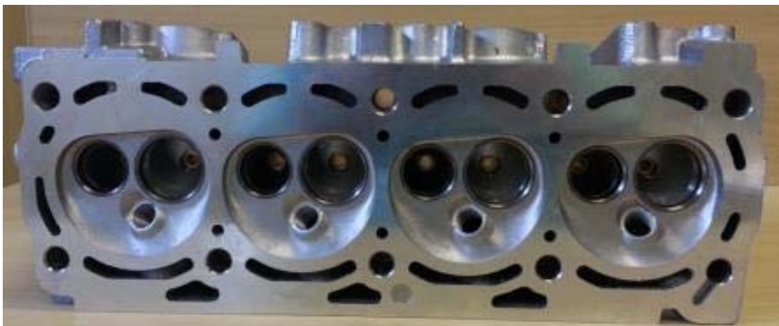
Figure 1. Engine head of eight pre-mounted valves
