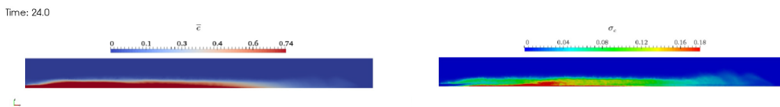
Figure 5. Concentration at time 24 in a longitudinal center channel cut
