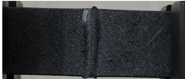
Figure 2. Standard texture necessary for the digital image correlation application.
