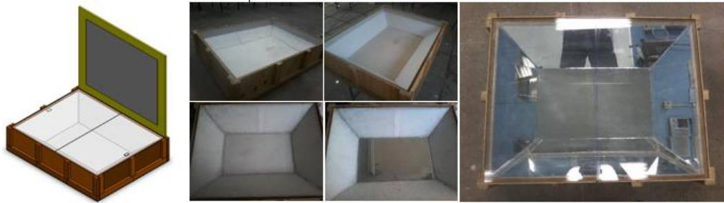
Figure 1. Sketch and steps of the construction of the mirrored oven.
