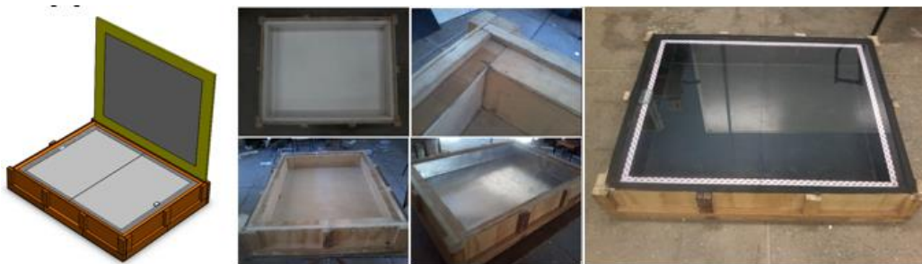
Figure 2. Sketch and some steps of the construction process of the dark oven.
