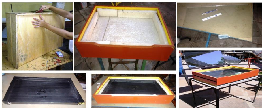
Figure 1. Manufacture and assemble processes of the studied solar oven
