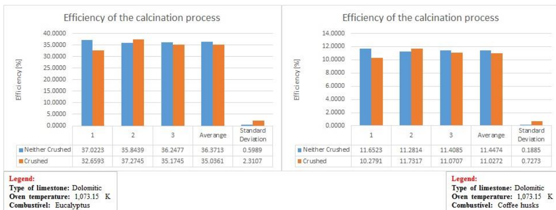
Figure 2: Calcination process efficiency for the method of the loss on ignition for the dolomitic limestone to 1,073.15 K.
