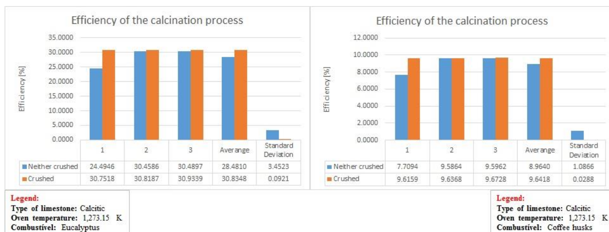
Figure 3. Calcination process efficiency for the method of the loss on ignition for the calcitic limestone to 1,273.15 K.
