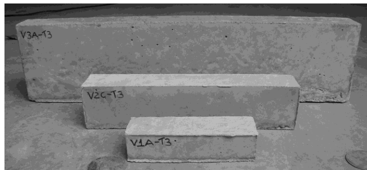
Figure 4. Different size concrete beams
