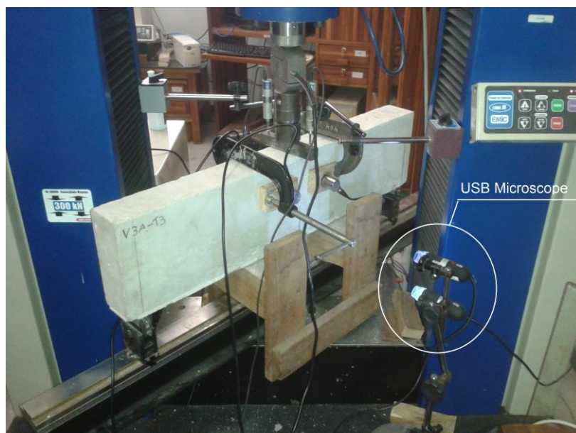
Figure 5. EMIC DL 30000 servo-hydraulic machine and USB microscope 800x
