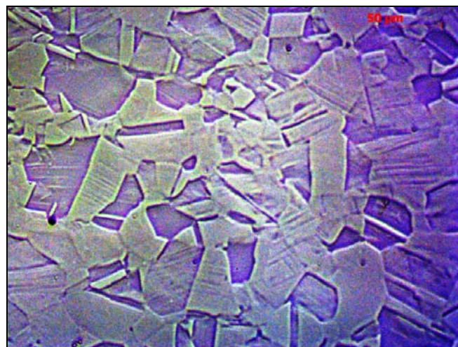
Figure 2. Optical microscope image of the microstructure of the femoral plate stainless steel without etching
