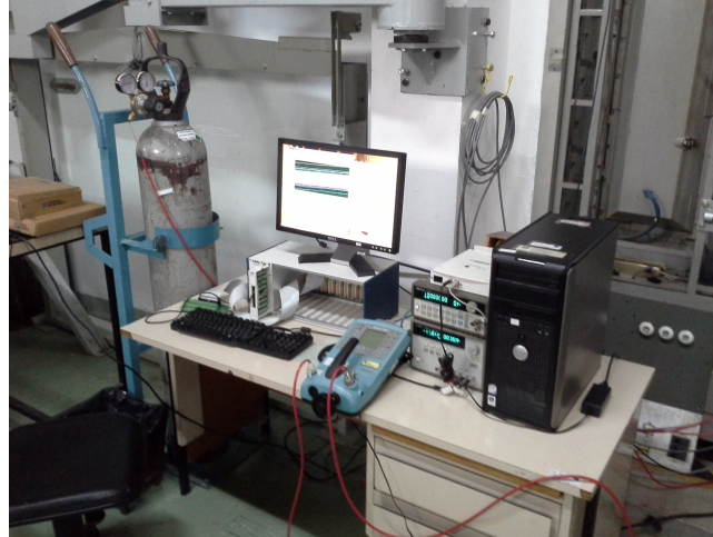
Figure 7. Standard instrument used to calibrate the pressure scanners.
