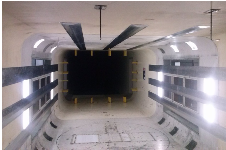
Figure 2. TA-2 test section instrumented with pressure taps in aluminum slats. Upstream of the flow we can see two Pitot tubes on the ceiling.
