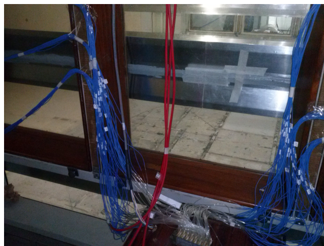
Figure 6. Tubing connecting the pressure taps to instrumentation.
