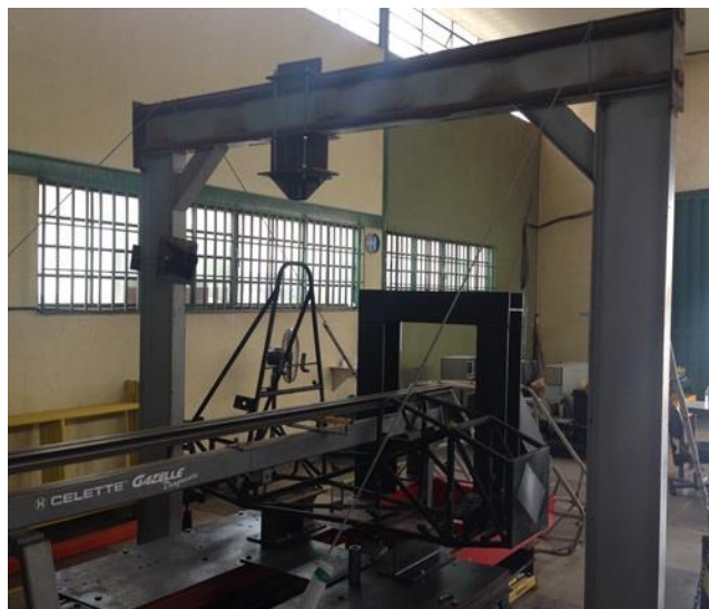
Figure 8. Chassis testing table
