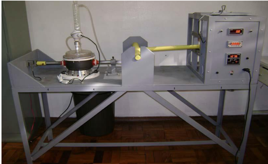
Figure 2. Device for CST constant load test.
