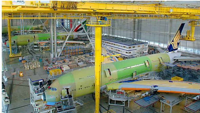
Figure 2. Final assembly line of A380. (source: Airbus, 2015)
